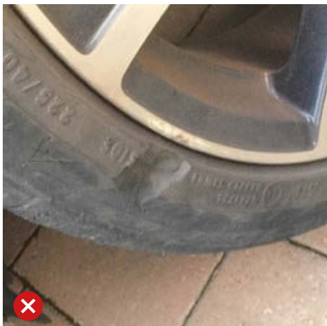
Tyre side wall damage is not acceptable.
