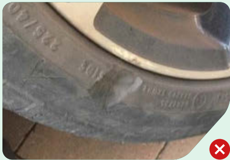
Tyre sidewall damage is not acceptable.
