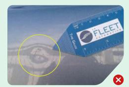
Dents over 15mm in diameter, or any dents to the roof or swage line on any panels, are not acceptable.
