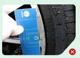
Scuffs to wheels totalling up to 50mm on the total circumference of the wheel trim, and on alloy wheels, are acceptable.
