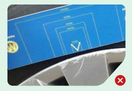
Scuffs to wheels totalling up to 50mm on the total circumference of the wheel trim, and on alloy wheels, are acceptable.
