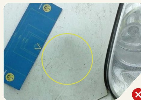
Dents over 15mm in diameter, or any dents to the roof or swage line on any panels, are not acceptable.
