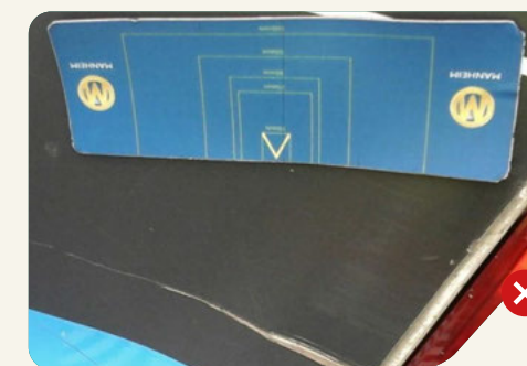
Scratches and abrasions over 25mm are not acceptable. Any scratch where the primer or base metal is shown will also be charged.
