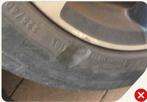
Tyre sidewall damage is not acceptable.
