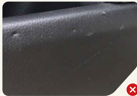
Holes to the interior upholstery and trim are not acceptable.
