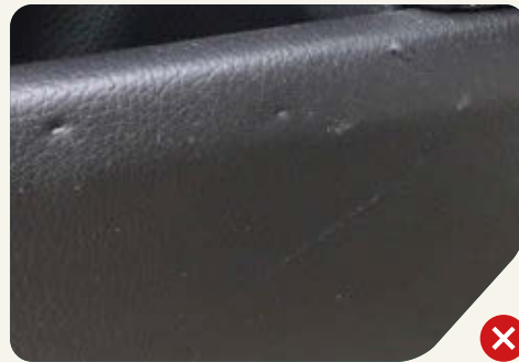
Holes to the interior upholstery and trim and not acceptable.
