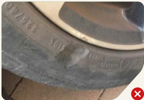
Tyre sidewall damage is not acceptable.
